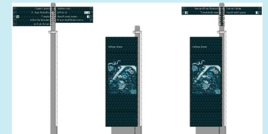
All components are physically and visually robust, taking their cue from Bristol's architecture and industry. Designed as a visible expression of the city's character – strong, creative, contemporary but not faddish – they are made of stainless steel, powder-coated mild steel and vitreous enamel panels to blend with the cityscape and give long-lasting, low-maintenance quality.
